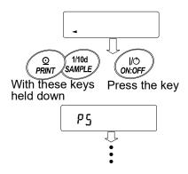
4 Press the PRINT key. Then the balance displays the function switches.
