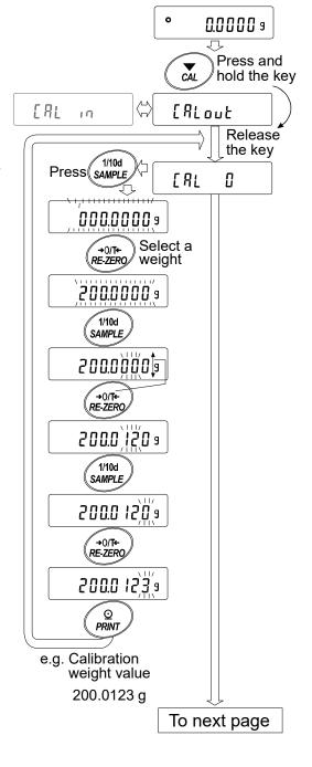
5 Confirm that there is nothing on the pan and press the PRINT key. The balance measures the zero point. Do not allow vibration or drafts to affect the balance.
