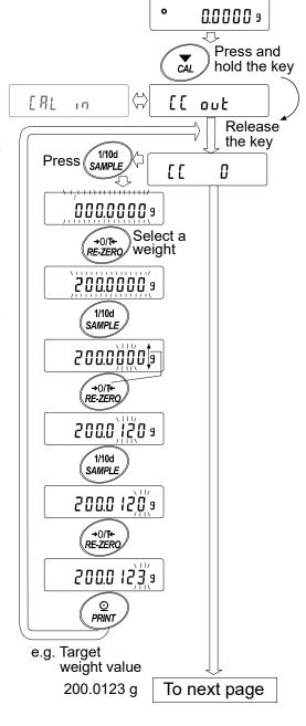
5 Confirm that there is nothing on the pan and press the PRINT key. The balance measures the zero point and displays the measured value. Do not allow vibration or drafts to affect the balance.
