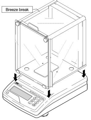
Secure the breeze break to the main unit using two screws provided with the breeze break.
